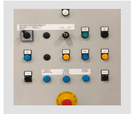
OPERATING PANEL Modern user-friendly operating panel with status indicators and commands for bale ejection and manual operation.
