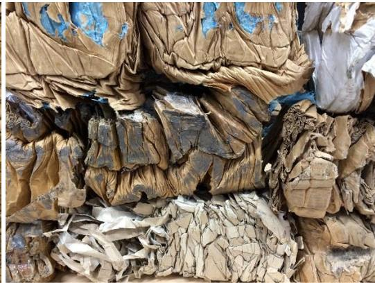
Close up on dense briquettes from a briquette press
