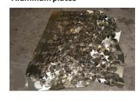
Scrap blister packs from the pharmaceutical industry is another type of material that is easy to briquette with good results in Brickman
